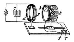
Figure 1. Tesla's WPT prototype.
