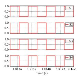
**Figure 7.** Switching signals of the inverter.
