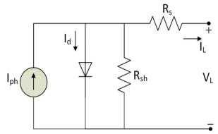
Figure 4. Circuit scheme of a PV cell.
