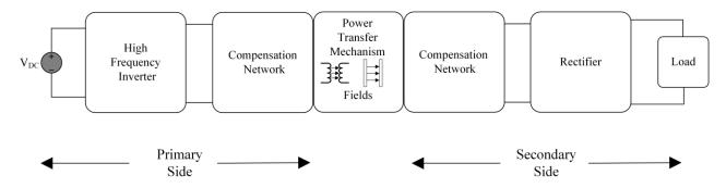
Figure 2. The typical configuration of a WPT system.
