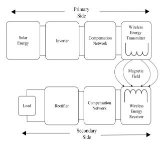
Figure 3. Solar energy-based IPT system.
