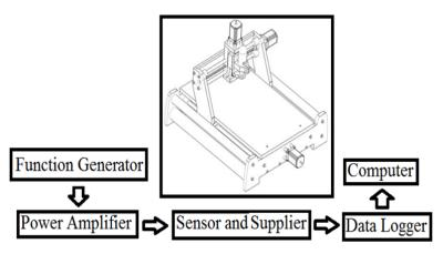
Figure 2. Scheme of magnetic measurement system
