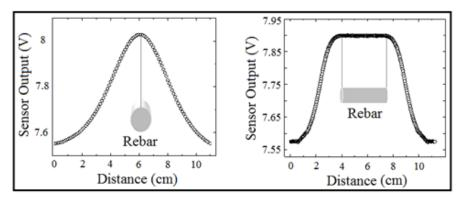
Figure 3. Rebar signals
