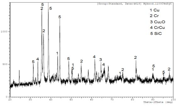
Figure 8. XRD analysis results of Cu-Cr-%4SiC composite at 1100°C
