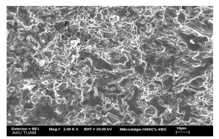
Figure 4. SEM view of Cu-Cr-4SiC composite 1000°C
