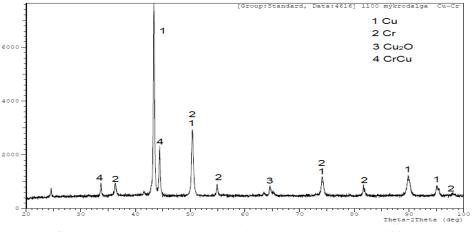
Figure 7. XRD analysis results of Cu-Cr composite at 1100°C
