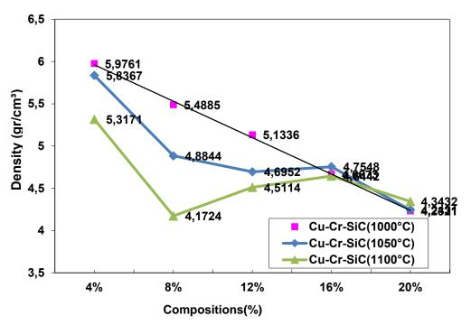
Figure 1. The density change with respect to sintering temperature
