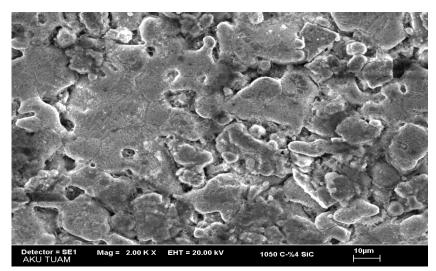
Figure 5. SEM view of Cu-Cr-4SiC composite 1050°C
