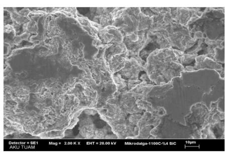
Figure 6. SEM view of Cu-Cr-4SiC composite 1100°C
