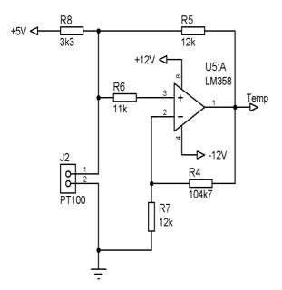
Fig. 5. The schema of PT100 amplification circuit
