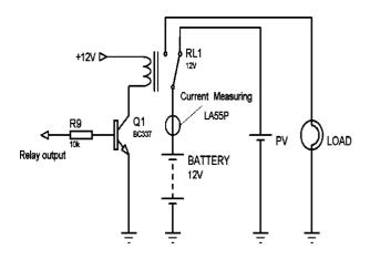
Fig. 4. Load and battery switching circuit
