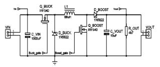
Fig. 2. The schema of buck-boost controller
