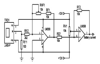
Fig. 7. Current to voltage converter circuit
