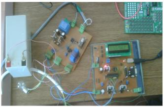
Fig. 10. The circuit of charge controller for PV panel
