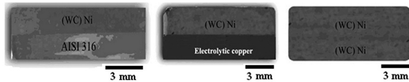
Fig. 3. The diffusion bonded specimens of (WC)Ni-AISI316, (WC)Ni-Cu and (WC)Ni-(WC)Ni (from left to right)
