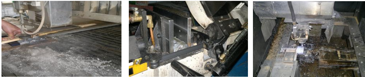
a) Cutting with water jet
