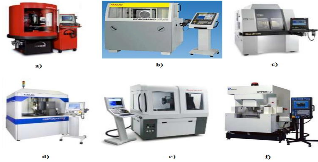
Resim 2.2 Çeşitli ticari mikro freze makineleri; a) Kern Micro (Wu 2012, İnt. Kyn. 10), b) Fanuc Robonano \alpha -0iB (Wu 2012, İnt. Kyn. 11), c) Sodick AZ250L (Wu 2012, İnt. Kyn. 12), d) Kuglar Micromaster (Wu 2012, İnt. Kyn. 13), e) Moore Nanotech 350UPM (Wu 2012, İnt. Kyn. 14), f) Makino Hyper2J (Wu 2012, İnt. Kyn. 15).
