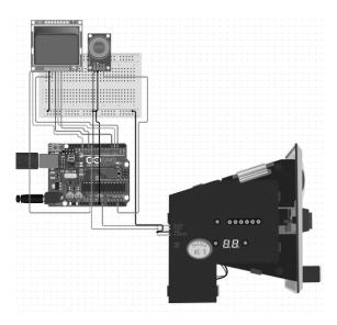
Figure 1. Alcoholmeter circuit diagram
