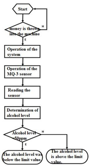
Figure 2. System working algorithm
