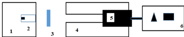
Fig.3: Experimental Set Up (1: lead shield, 2: X-ray source, 3: glass sample, 4: lead shield, 5: detector, 6: PC monitor).
