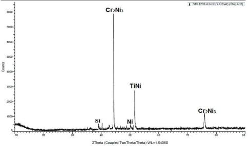
FIGURE 6. The XRD analysis (Ni-Cr-4Ti)%10NF composite Sintered in tube furnace at 1200°C
