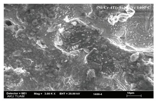
FIGURE 4. SEM view of (Ni-Cr-4Ti)-%10NF composite 1400°C
