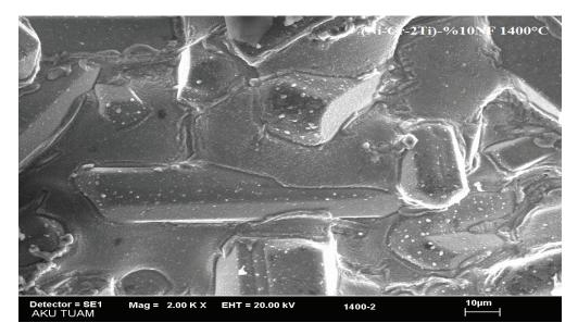
FIGURE 3. SEM view of (Ni-Cr-2Ti)-%10NF composite 1400°C
