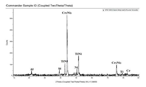
FIGURE 5. The XRD analysis (Ni-Cr-2Ti)%10NF composite Sintered in tube furnace at 1200°C
