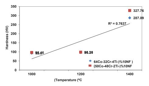
FIGURE 2. The micro hardness tests results from sintered specimens treated at different temperatures
