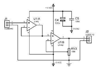
Figure 6.Operational trans conductance amplifier.
