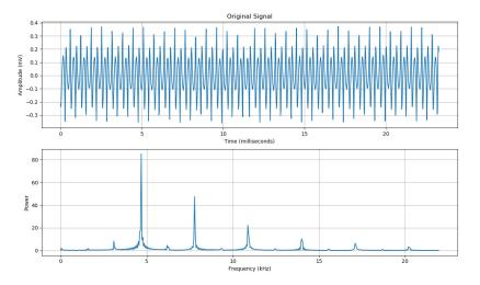
Figure 12. 38 KHz sampled MPS signal and FFT
