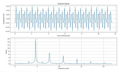
Figure 11. 16 KHz sampled MPS signal and FFT
