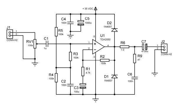
Figure 4. Current drive power amplifier with TDA2050
