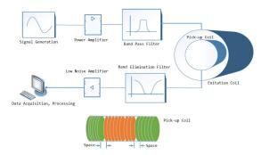
Figure 8. The signal flow of the system.
