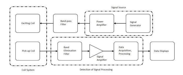
Figure 2. The system schematic of magnetic nanoparticles detection.
