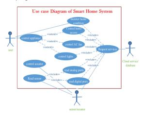
Figure 3 Use case diagram showing smart home architecture (Int ref. 1).
