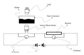
**Figure 1.** The schematic representation of the designed measurement system
