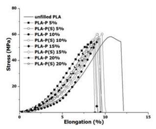
Figure 2. Tensile curves of PLA and composites
