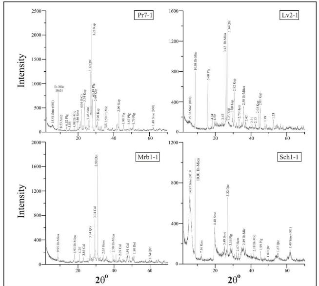
Figure 3. The whole rock XRD diagrams of representative samples from the BAYATCIK-1 well. (Sme): Smectite, (Ilt-Mic): Illite-Mica, (Amp): Amphibole, (Plg): Plagioclase, (Kao): Kaolinite, (Qtz): Quartz, (Ksp): Alkali feldspar, (Hem): Hematite, (Cal): Calcite, (Dol): Dolomite
