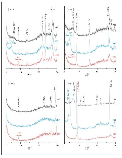
**Figure 4.** Representative XRD patterns of clay fraction of samples from the Bayatcık-1 well. Key to the symbols: (AD): Air dried, (EG): Ethylene glycolated, (550): Heated at 550 oC.
