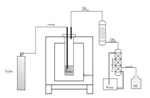
**Figure 4.** A diagram of the bench-scale pyrolysis reactor (Shuaib and Mativenga 2016).
