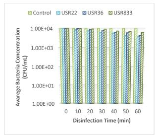
Figure 3. The result of US disinfection according to ultasonic frequency
