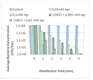
**Figure 5**. The result of synergistic US and Ag<sup>+</sup> disinfection
