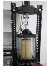
Figure 3. Resilient modulus test
