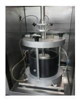
Figure 5. Triaxial cyclic compression test for foam bituminous mixture
