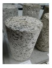
Figure 4. Unconfined compressive strength samples
