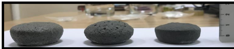
Fig. 5. The front-view of foamed glass samples produced (from left to right: S1, S2 and S3).
