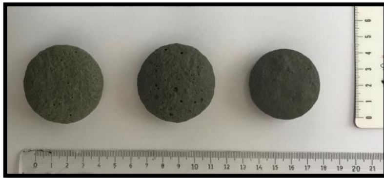
Fig. 4. The top-view of foamed glass samples produced (from left to right: S1, S2 and S3).
