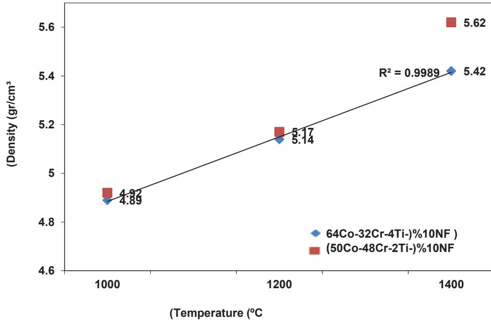
**FIGURE 1.** The density change with respect to sintering temperature
