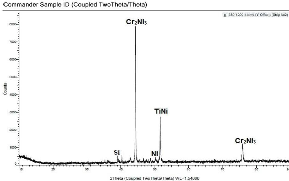
**FIGURE 6.** The XRD analysis (Ni-Cr-4Ti)%10NF composite Sintered in tube furnace at 1200°C
