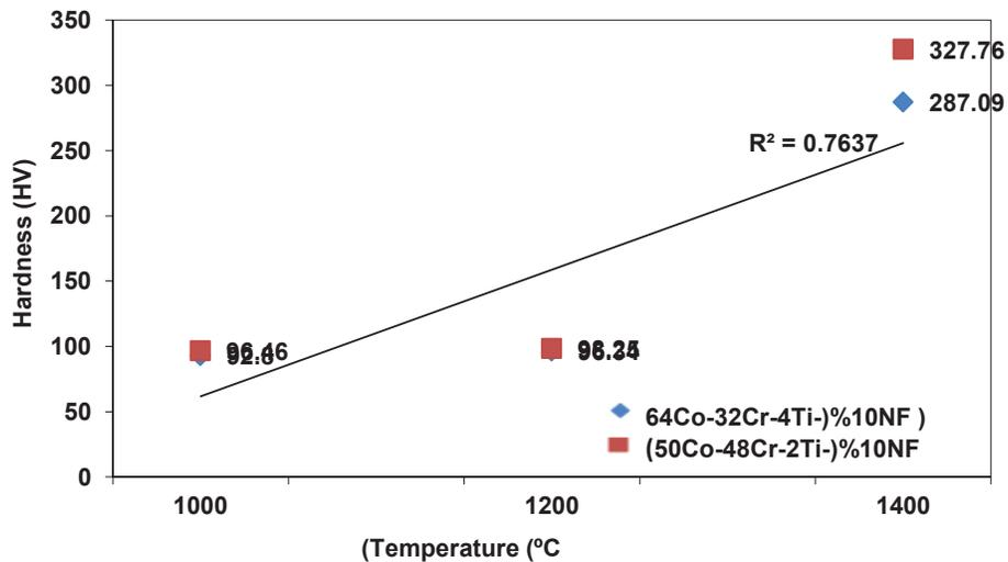
**FIGURE 2.** The micro hardness tests results from sintered specimens treated at different temperatures
