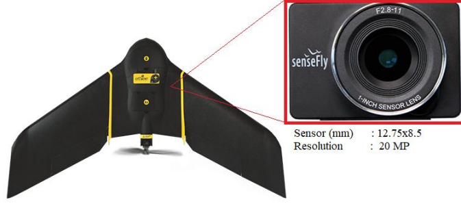
Şekil 4.3 Sensefly Ebee Plus İHA (İnt. Kyn.2).
