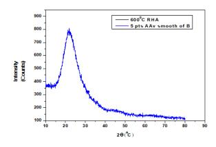
Figure 1. The Al-RHA composite of XRD peaks.
