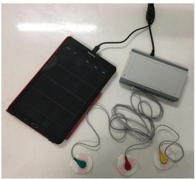
Figure 1. Prototype moduler ECG and EMG device.
